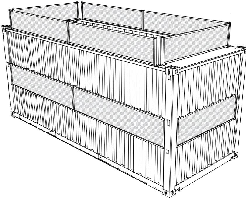
BioFiltro is proud to offer the Wiggler Room, a 20' shipping container which houses our patented biodynamic aerobic (BIDA®) technology. Providing two floors of treatment capacity, a single unit can meet the full wastewater needs of a boutique winery or be deployed as a fleet to provide modular and scalable solutions for larger wineries.
